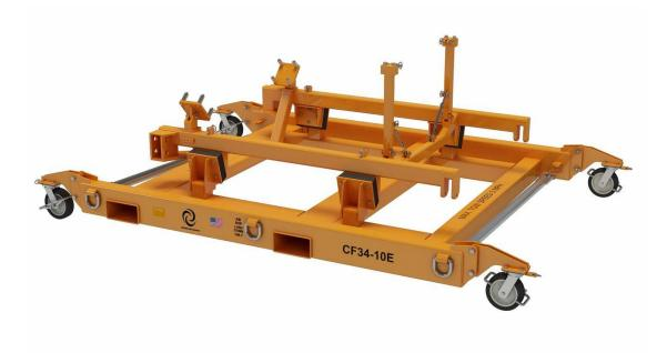
The NGCF3410E CF34-10E Air/Truck Shipping Stand is designed to transport the CF34-10E engine on an air ride trailer or the main deck of commercial freighters. The stand includes casters with swivel locks and brakes, towbars, Skydrol resistant paint, a shock isolation system to protect the engine from handling shocks and road vibration and ERJ-190 bootstrap interfaces.
